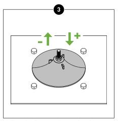
Adjust the flow rate by turning the cone: Up = less flow Down = more flow
