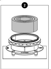
Pre-adjustment: remove the acoustic rings from the foam pack according to the desired flow rate. See the overview under "Calibrating flow rates". Leave at least the outer ring in place for an acoustic effect!
