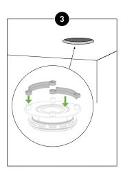
When mounting less than 20 cm from a wall or corner: mount the directional plates.
