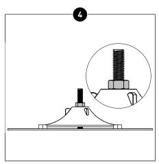
When the flow rate has been adjusted correctly, secure the cone by tightening the lock nut wit a spanner 10.
