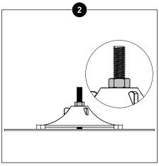
Loosen the lock nut with a spanner 10.
