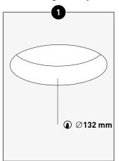
Cut out a hole in the plasterboard at the desired location. Make sure the surface is flat and even.
