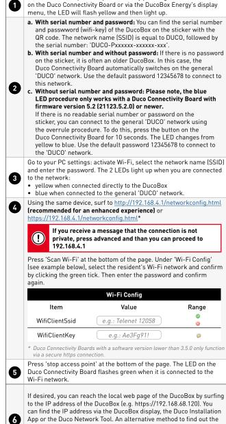
can find the IP address via the DucoBox display, the Duco Installation App or the Duco Network Tool. An alternative method to find out the IP address is to use MDNS discovery apps such as 'Discovery App' for iOS or 'MDNS Discovery' for Android devices. In these apps, look for an HTTPS connection over SSL/TLS.
