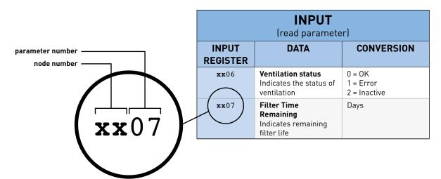
This allows all values to be read and controlled from the external control unit. There are specific parameters for each component.
