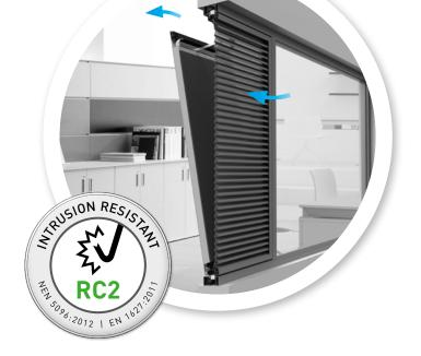
The DucoGrille NightVent is a glass replacement ventilation shutter (for glass thicknesses from 24 to 48 mm) that provides efficient cooling and ventilation of any building thanks to the supply of **large ventilation flow rates** (369 l/s\*m<sup>2</sup> at 2 Pa pressure difference).
